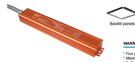
The HM series 8W LED emergency driver is designed for LED fixtures such as backlit panels and LED troffers. Rated to provide a minimum of 90 minutes of emergency illumination. When the AC power goes out, the emergency driver detects the AC power outage and automatically switch to the working emergency mode. When the AC power is restored, it starts re-charging.
